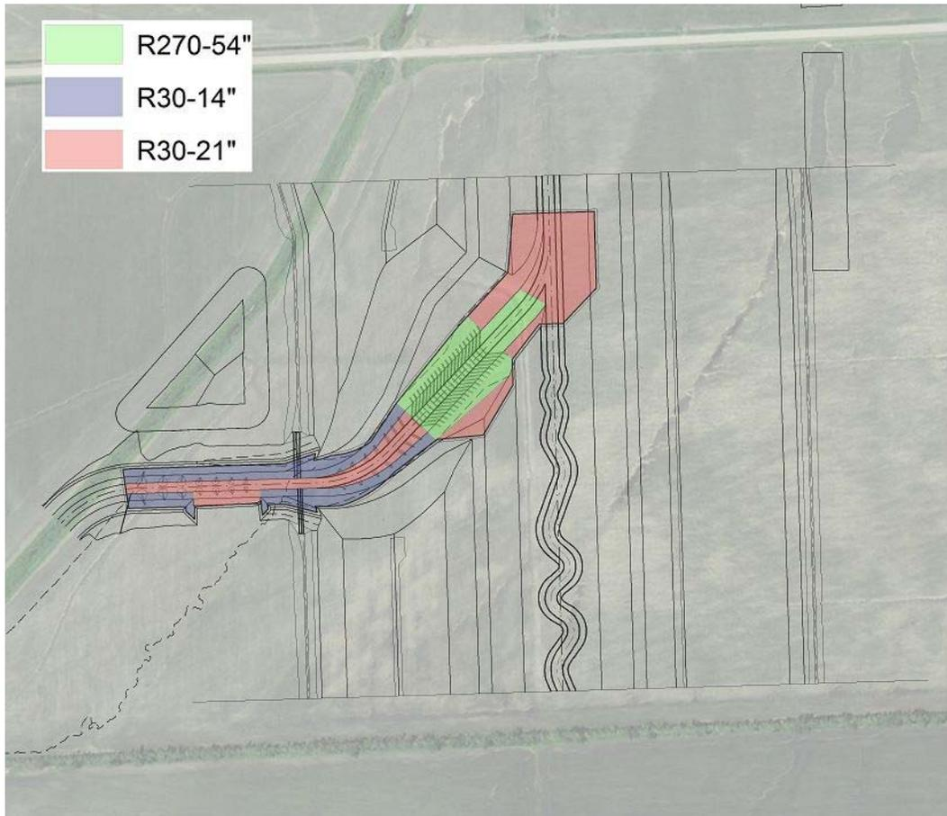
Figure C. 8 Plan View of Riprap Gradations and Thicknesses of the Lower Rush River Inlet Structure
