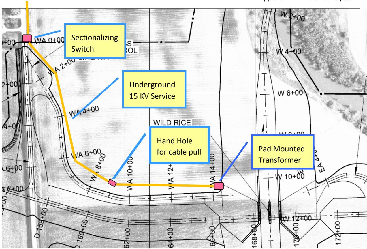
Figure H-2. Detailed Site Power Routing.
